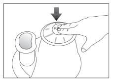
8 Turn the speed control and locking / unlocking button B to the Off position when you want to finish the operation.
